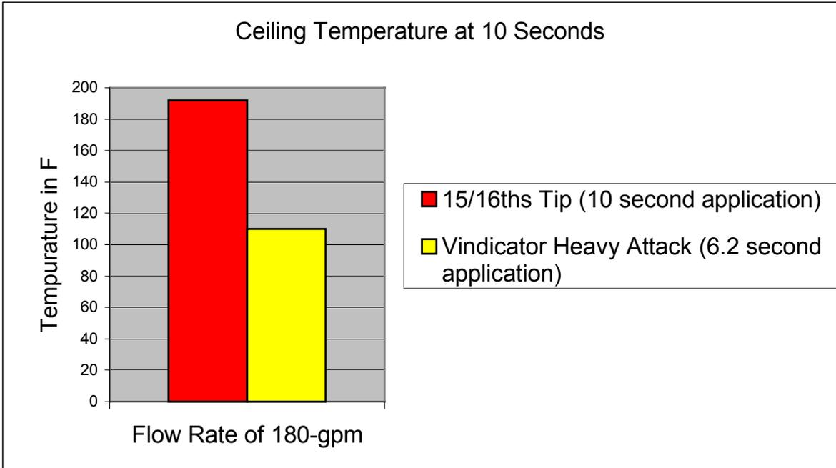
3. At the same Nozzle Pressure the Vindicator was able to bring the room temperature down 44% lower than the 15/16ths tip in the same amount of time.
